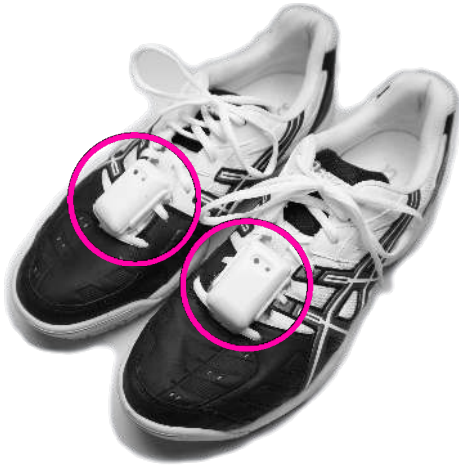
Fig. 3: Placement of two EXLs3 IMU sensors on shoes.
