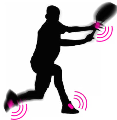
Fig. 1: Capturing coordination of hitting arm along with the footwork of the player with three IMUs.
