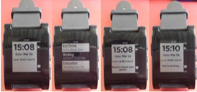
Figure 2. An illustrations of the screens that a user sees when labelling activity routines via the Pebble interface. On the initial screen, the start and stop buttons are shown. Upon pressing the start button via the selectors on the right of the watch, a selection screen is displayed to mark the current activity routine. The user receives a confirmation message after confirming the selection of an activity (third photo). Finally, the current marked activity is shown after a few minutes into the activity.
