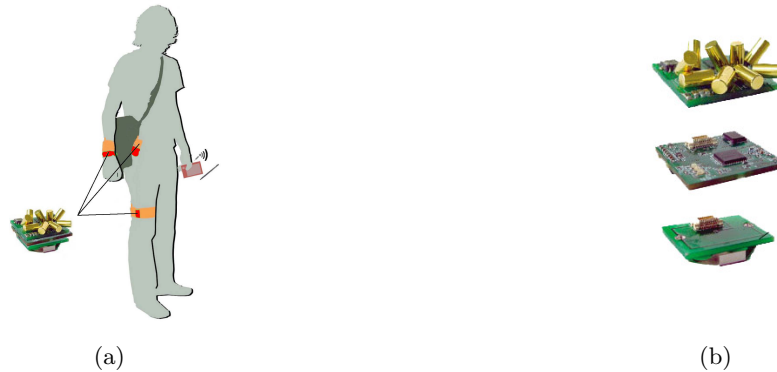
Fig. 3. Left: User wearing sensors on wrist, hip and thigh. Right: The sensor platform, consisting of the power supply (bottom), the BSN node for logging (middle) and the sensor board (top).
